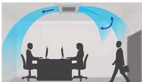
Individual louvers can be programmed separately. Adjust vertical airflow and louver position with UTY-RNRUZ Series Wired Remote Control.
