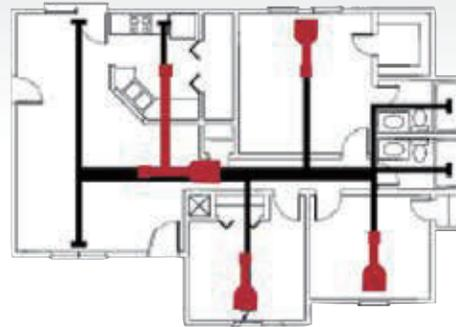
Thick black lines represent ducts of a central air system.
