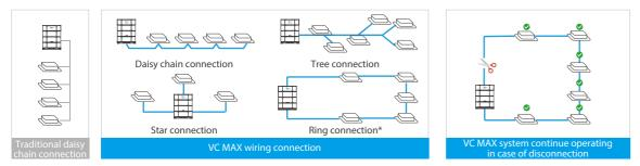
\*In ring connection, the communication wire must be connected polarized (M1 port to M1 port and M2 port to M2 port).
