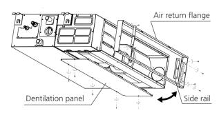
2. Stick the attached seal sponge as per the indicating place in the following fig, and then change the mounting positions of air return panel and air return flange.
