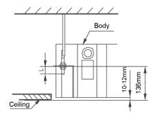
Locate the air conditioner firmly by wrenching the nuts after having adjusted the body's position well.
