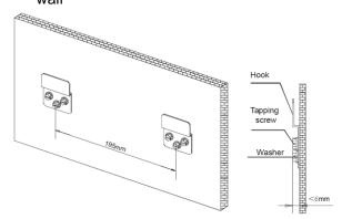
(The bottom of body can touch with floor or suspended, but the body must install vertically.)
