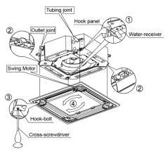
Tighten the screws under the panel hooks till the panel closely stick on the ceiling to avoid condensate water.
