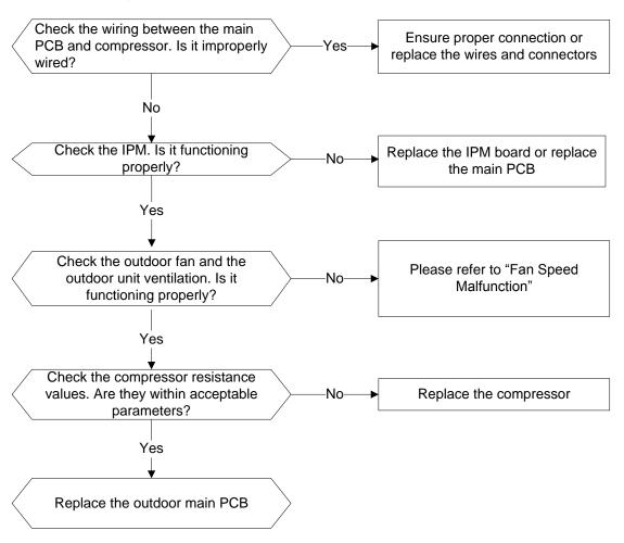
16.4.11 Outdoor IPM module temperature sensor malfunction diagnosis and solution (P7)
