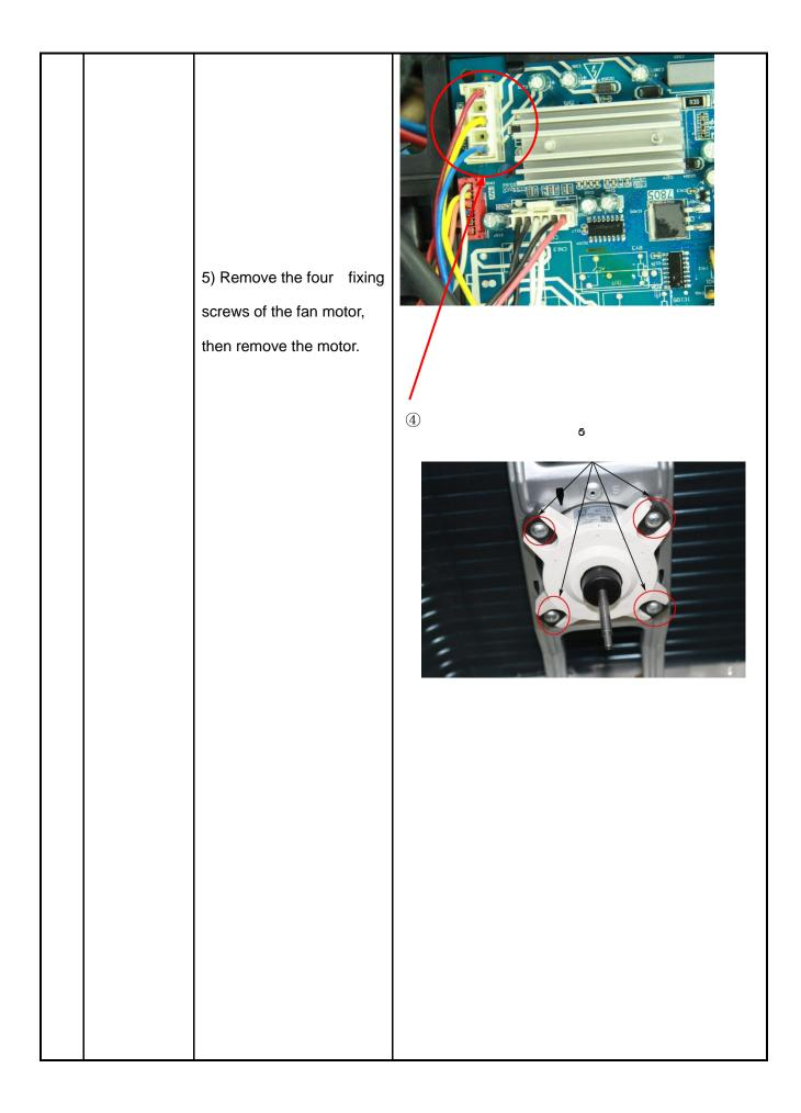
3 Electrical How to remove the parts electrical parts. 5) After finish work of item 1 and item 2, remove the connector for the compressor. 6) Pull out the two blue wires connected with the four way valve. 3) Pull out connectors of the condenser coil temp. sensor(T3),outdoor ambient temp. sensor(T4) and discharge temp. sensor(T5). 4) Disconnect the
