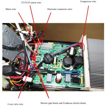
Disconnect the connector for fan motor
