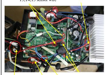
Electric pipe heater and Crankcase electric Heater wire
