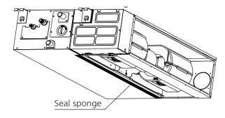
3. When installing the filter mesh, fit it into the flange inclined from air return opening, and then push up.
