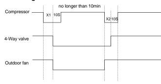
15.4.3.5 Evaporator coil temperature protection
