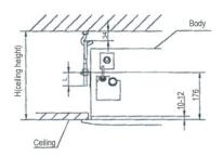
Locate the air conditioner firmly by wrenching the nuts after having adjusted the body's position well.
