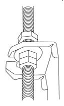
Mount the indoor unit onto the hanging screw bolts with a block. Position the indoor unit flat using a level indicator to prevent leaks.
