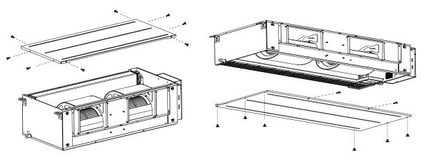
The air outlet flange is isolated from either top panel or base panel, which makes the maintenance much easier when connecting duct.
