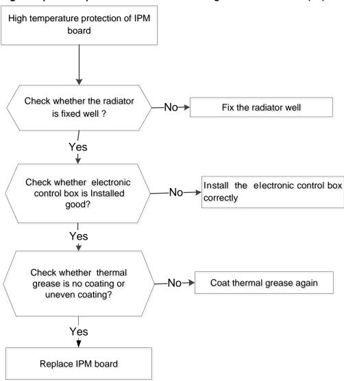
16.4.10 Inverter compressor drive error diagnosis and solution(P4)
