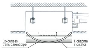
Adjust the position to ensure the gaps between the body and the four sides of ceiling are even. The body's lower part should sink into the ceiling for 10~12 mm. In general, L is half of the screw length of the installation hook.
