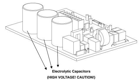
For other models, For other models, connect a discharge resistor (approx.100 $\Omega$  40W) or a soldering iron plug between the + and - terminals of the electrolytic capacitor on the opposite side of the outdoor printed circuit board (PCB).
