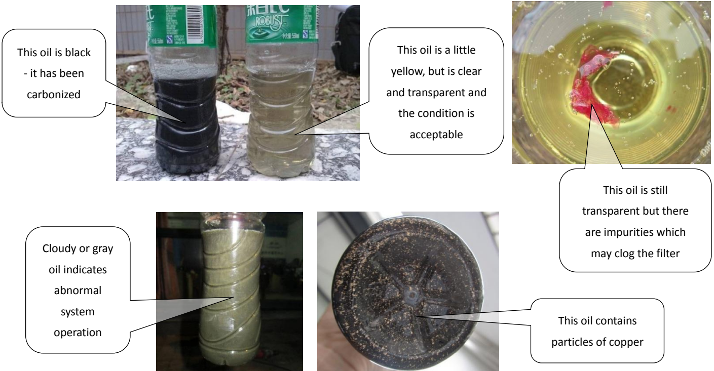
Figure 5-4.16: Inspecting compressor oil
