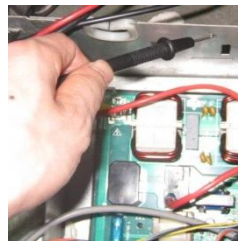
Figure 5-4.7: Measuring resistances between compressor terminals and ground
