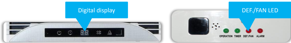
Figure 4-1.3: Indoor unit digital displays and LED indicators
