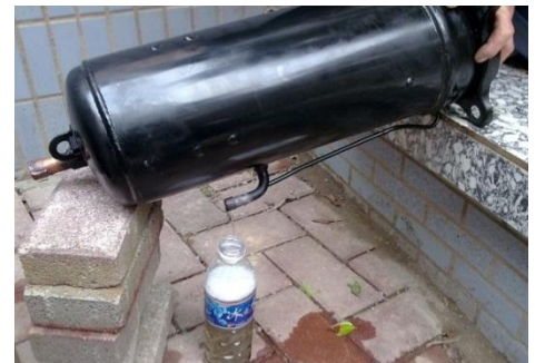
Figure 5-4.14: Draining oil from a compressor
