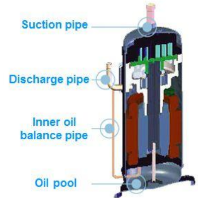
Figure 5-4.15: Compressor piping
