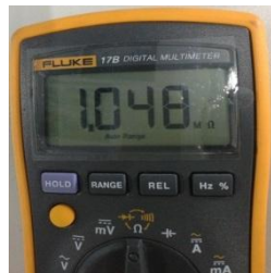
Figure 5-4.6: Measuring resistances among compressor terminals
