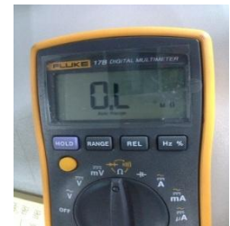
Figure 5-4.7: Measuring resistances between compressor terminals and ground
