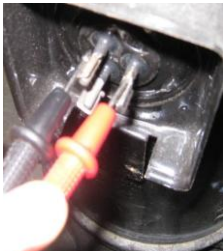
Figure 5-4.6: Measuring resistances among compressor terminals
